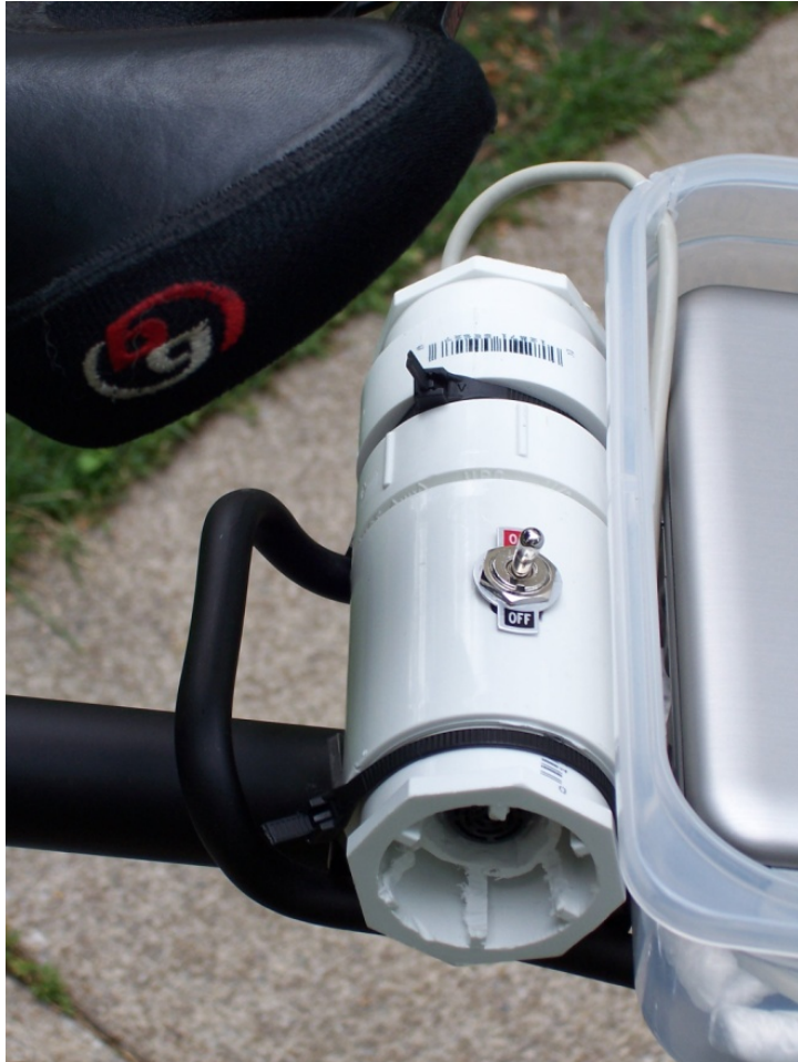
6 7 FIGURE 5: Ultrasonic Lateral Distance Sensor Detail View
